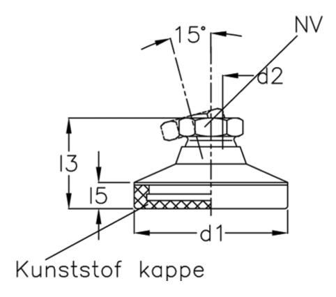
d1 = 32 d2 = 10 l3 = 24.5 l5 = 6.5 NV = 15 Static load (N) = 11 t min = 10.5
